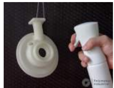
Figure 5. Spray isopropyl alcohol on the PolyCast™ pattern
