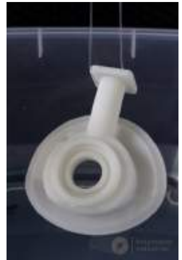
Figure 4. Dip the PolyCast™ pattern into isopropyl alcohol
