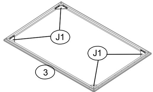
1. When diagonal measurements are equal, the frame is square.
