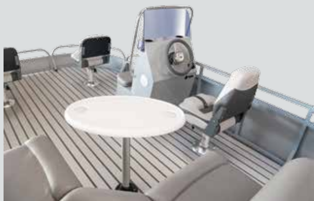
Spacious deck with fishing area, equipped with rotating and folding seats, rod-holders and other appliances for successful fishing, as well as seating area with a removable table with cup holders
