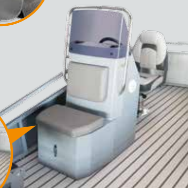
Welded aluminum steering console with forward seat and locker
