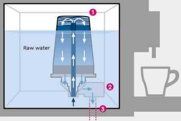
BWT bestcup PREMIUM filter cartridges **1** can be used easily in the tanks of a wide range of coffee and espresso machine via an adapter.
