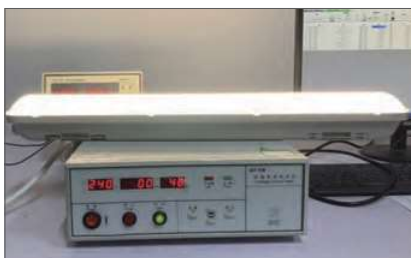
High-voltage Insulation Test
