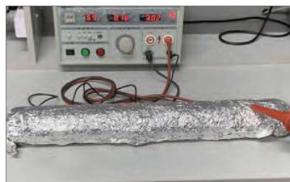
Leakage Current Test
