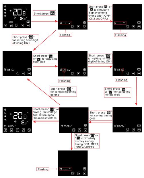
Notes: If there is no operation for 20 s, the system will automatically memorize user's setting, and return to the main interface; If the timing symbol and entire time digits flash at the same time, click "" for returning to the main interface.
